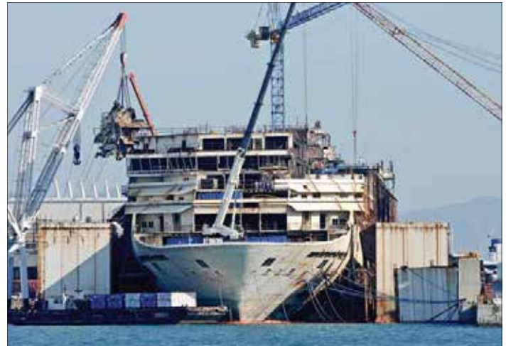
(Top) The stabilized wreck of the Costa Concordia enters the port pushed by tugboats. (Right) Once in dry dock at the San Giorgio shipyard, the dismantling of the Costa Concordia began. Upper decks were removed until only the hull remained. Photos by Riccardo Arata/Shutterstock.com.
