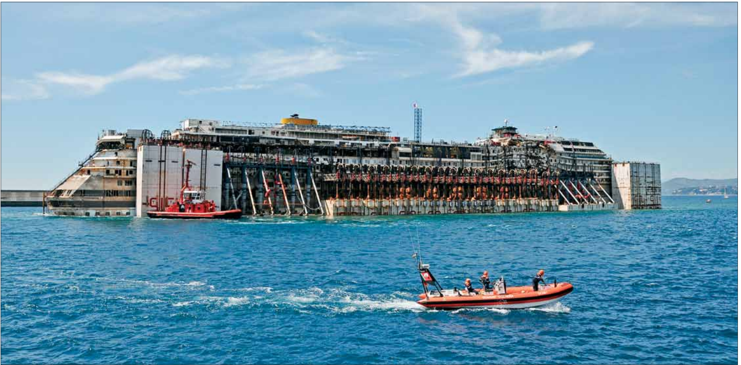
(Top) The stabilized wreck of the Costa Concordia enters the port pushed by tugboats. (Right) Once in dry dock at the San Giorgio shipyard, the dismantling of the Costa Concordia began. Upper decks were removed until only the hull remained. Photos by Riccardo Arata/Shutterstock.com.
